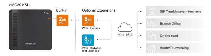
iPECS eMG80 is a hybrid TDM/IP system ideal for cost effective solutions. With its modular and flexible design, businesses can easily and affordably expand into Unified Communications and more sophisticated enterprise applications.
